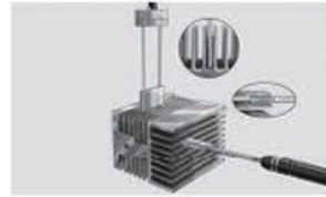
Surface temperature measurement of heat sink
