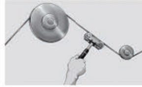
Temperature measurement of moving wire 测量移动钢丝温度
