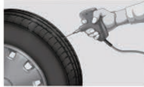
Internal temperature measurement of rubber 测量橡胶材预热温度
