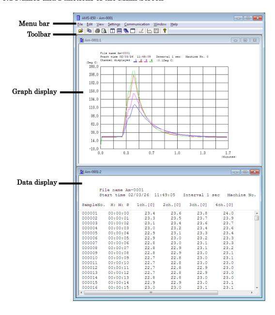
Menu bar: Allows you to set functions and perform measurements.
