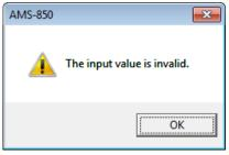
(4) If the measuring instrument cannot be communicated with Confirm the following: FL-2400 is powered on; communication cables are properly connected; and communication ports are correctly set.
