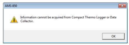
(5) If the measuring instrument is not connected to your PC Check whether the communication port on your PC is set to USB, or whether there are any problems with the communication port settings.
