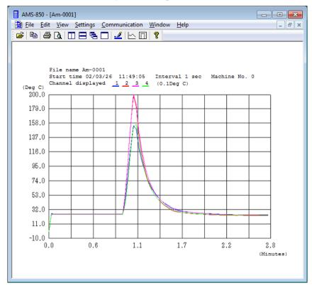
• You can use the toolbar to switch between graph display and data display.
