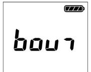
If the sensor burns out or is not coupled, the Burnout display appears shown as left.
