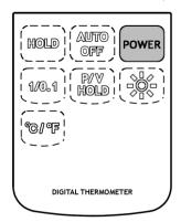
Press the POWER key to turn power ON and all segments appear on the display for 1 second, and start measurement as be shown below.
