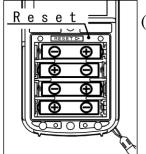
(3) After setting battery cells, press the Reset switch.
