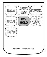
Press the P/V HOLD key to enter P/V Hold mode that the maximum value, the minimum value and the present value are displayed simultaneously.
