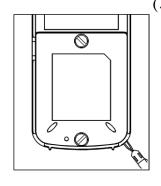
(4) Reattach the battery housing cover, tighten the two screws and press the edges of the battery housing cover firmly.
