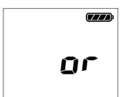
If the temperature exceeds the measurable range during measuring, the Over range display appears shown as right.
