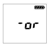
The over range display does not damage the instrument, however the sensor will be exhausted. Avoid the sensor to the place in measurable temperature.
