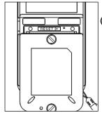
(1) Remove the two screws and detach the battery housing cover.
