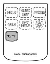
Press the °C/° F | key to change the temperature unit of the displayed temperature.
